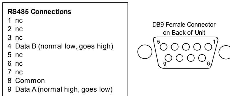
Figure 5.4: RS485 Wiring Connections
