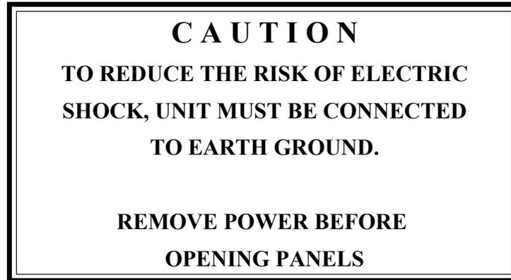
1. To properly operate this power supply, only electric cords with a 3-prong grounded system are to be used.
