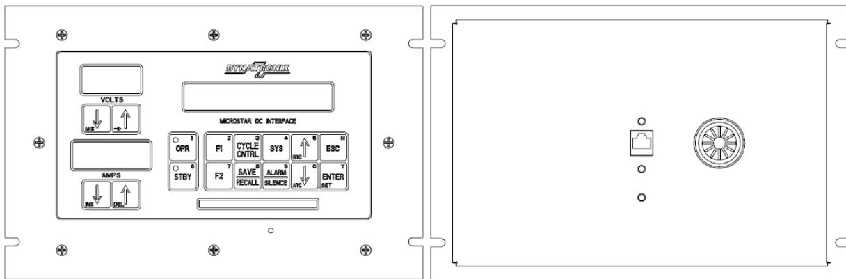
Figure 5.3: Remote MicroStar Panel: Front & Rear Views
