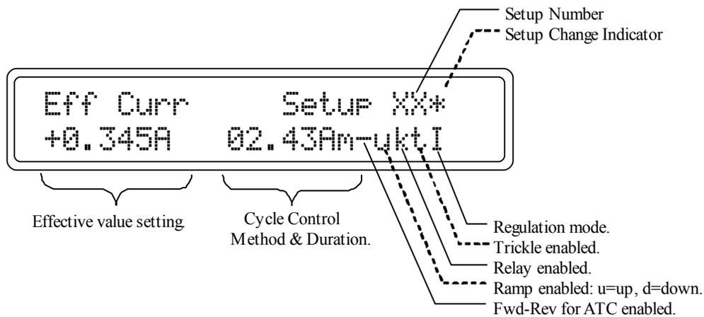
**Figure 6.28: Main Screen Indicating the Setup Parameters**
