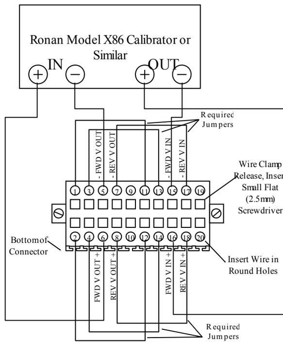
**Figure 7.4: Analog Calibration Connections - Forward Voltage Channel**
