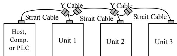
Figure 5.5: RS485 Host Connections with 3 Units
