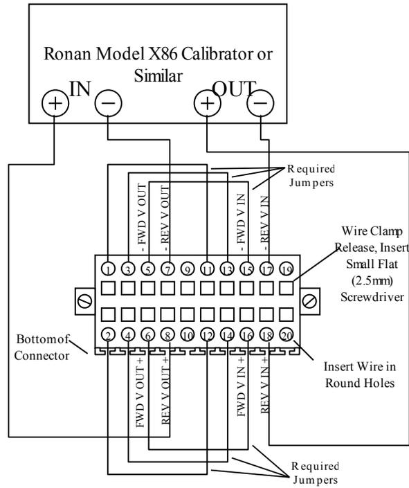
**Figure 7.5: Analog Calibration Connections - Reverse Voltage Channel - (option)**
